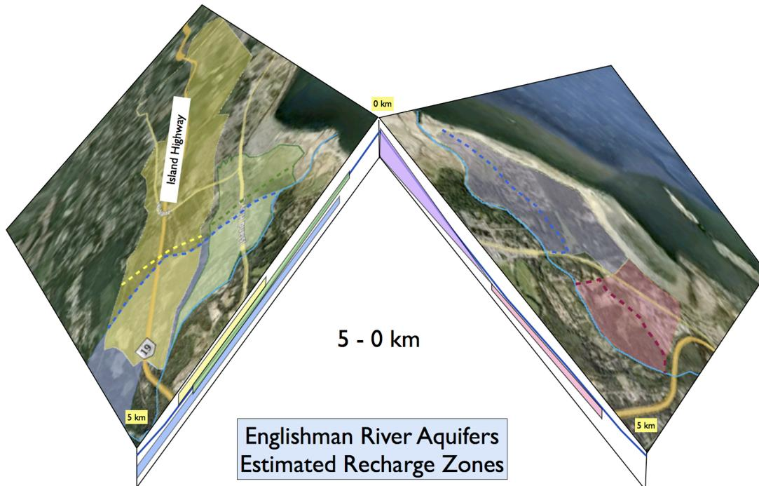
**Figure 26: Estimated recharge zones of overburden aquifers contributing to ER, 5 km to 0 km**
