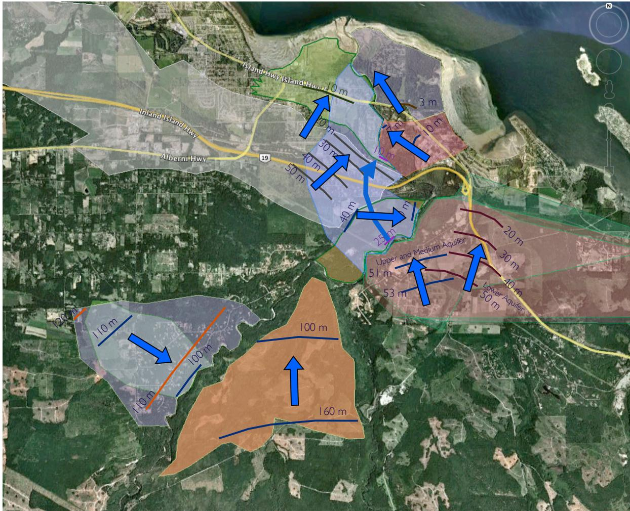
Figure 19: Estimated hydraulic gradients in overburden aquifers
