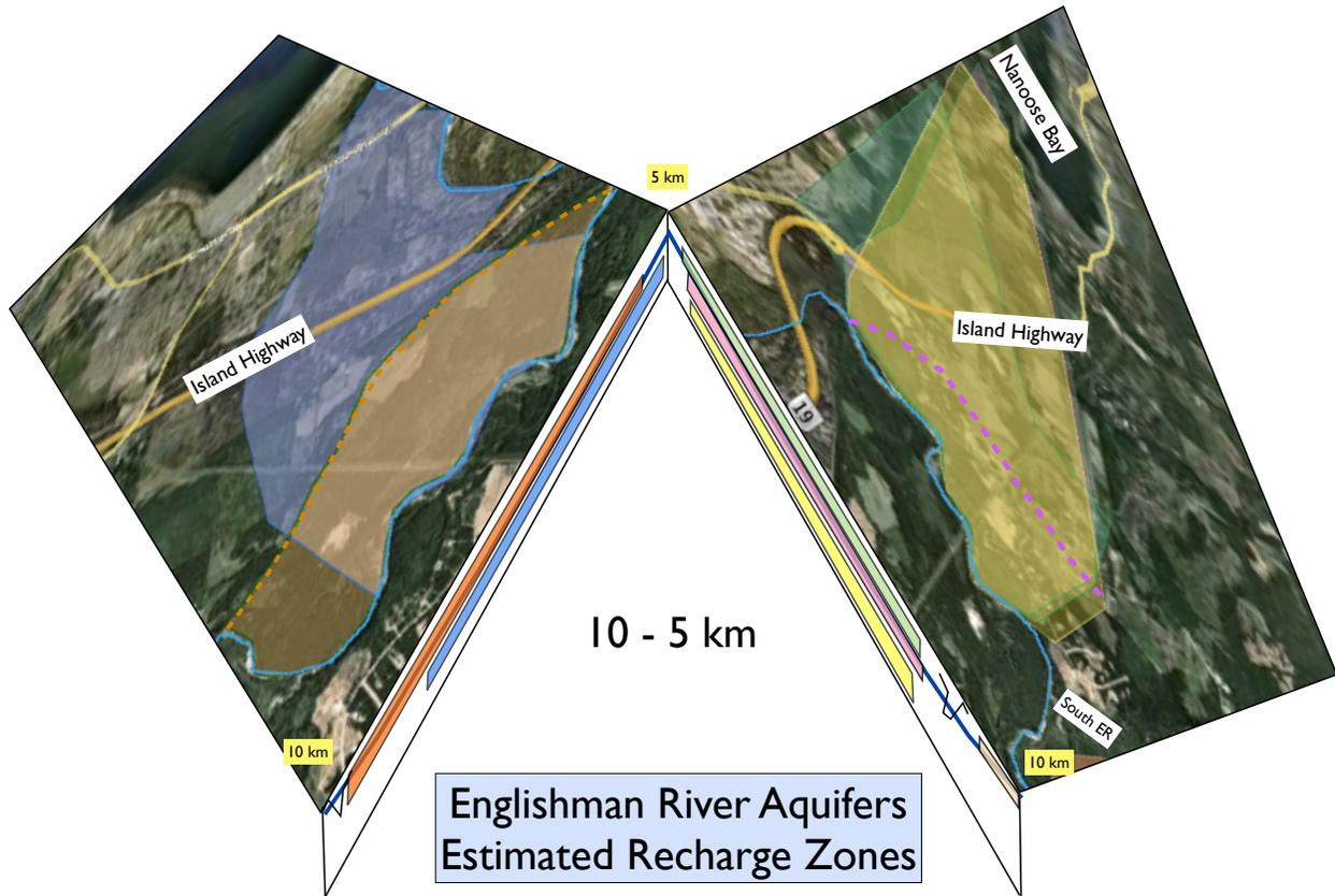
Figure 25: Estimated recharge zones of overburden aquifers contributing to ER, 10 km to 5 km
