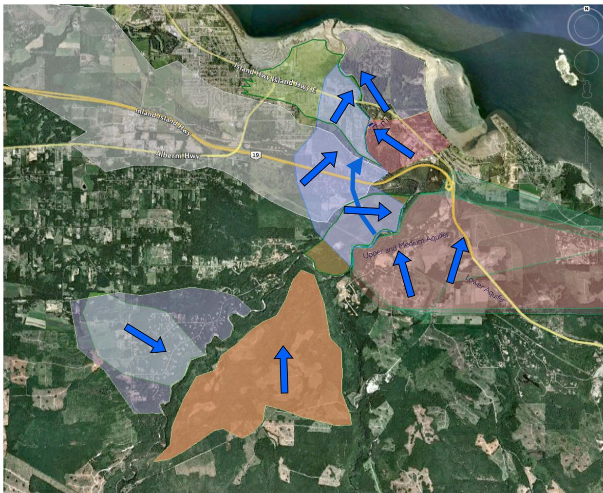
Figure 17: General groundwater directions in overburden aquifers in ER lower watershed
