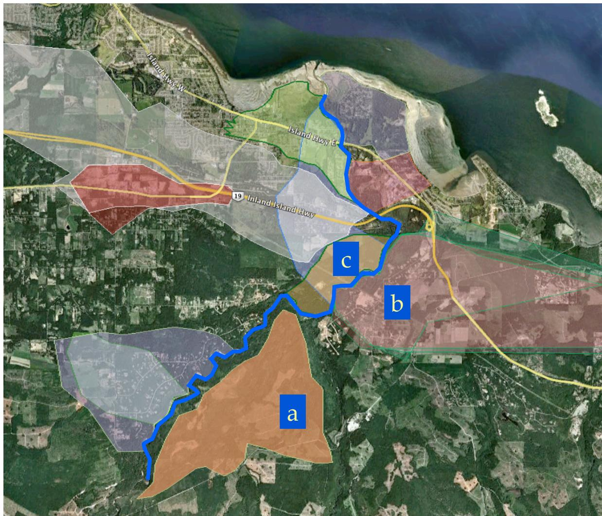
**Figure 12: Estimated footprints of overburden aquifers in contact with the ER**
