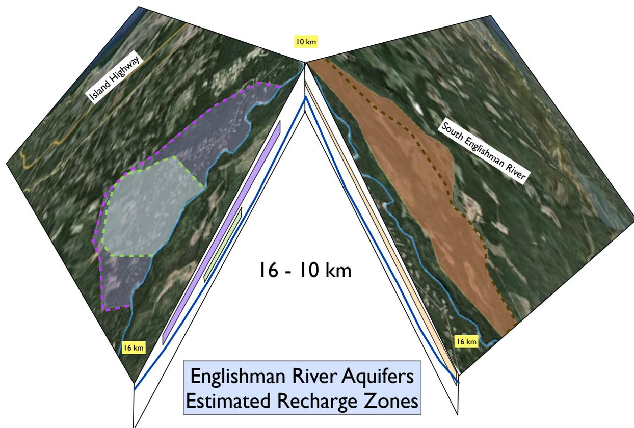
Figure 24: Estimated recharge zones of overburden aquifers contributing to ER, 16 km to 10 km
