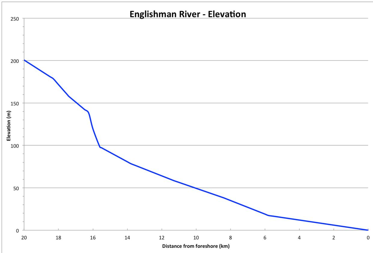
**Figure 11: Profile of lowest 20 km of ER main stem**
